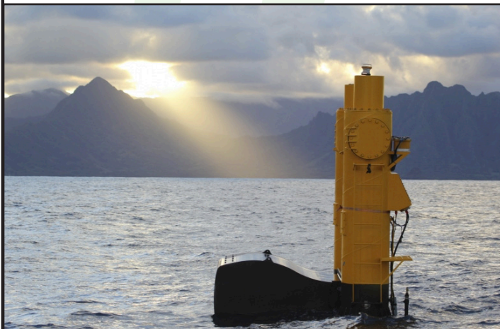
Azura is a wave power device currently being tested in Hawaii
